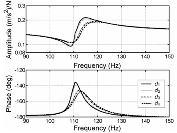
**Fig. 11:** Tuning of the damping ( $d_{avc} = d_i$ ,  $d_1 < d_2 < d_3 < d_4$ ;  $k_{avc} = k_2$ )
