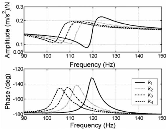
**Fig. 10:** Tuning of the stiffness ( $k_{avc} = k_i$ ,  $k_1 > k_2 > k_3 > k_4$ )
