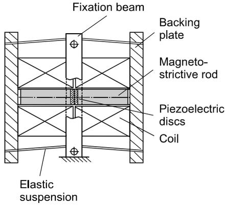
**Fig. 1:** Construction of tunable DVA
