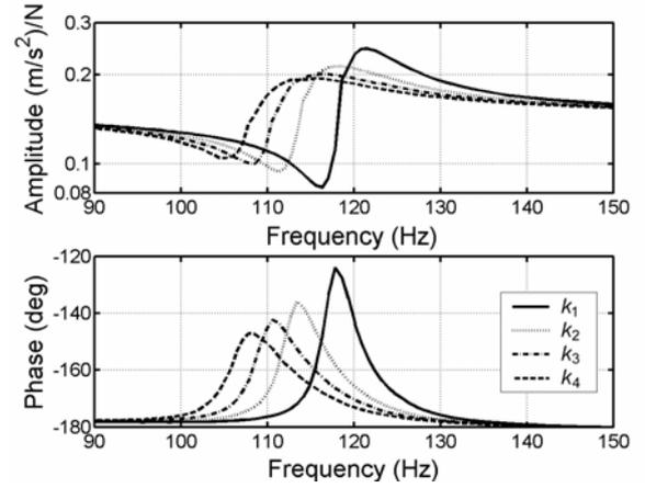
**Fig. 7:** Tuning of the stiffness ( $k_{\text{avc}} = k_i$ ,  $k_1 > k_2 > k_3 > k_4$ )
