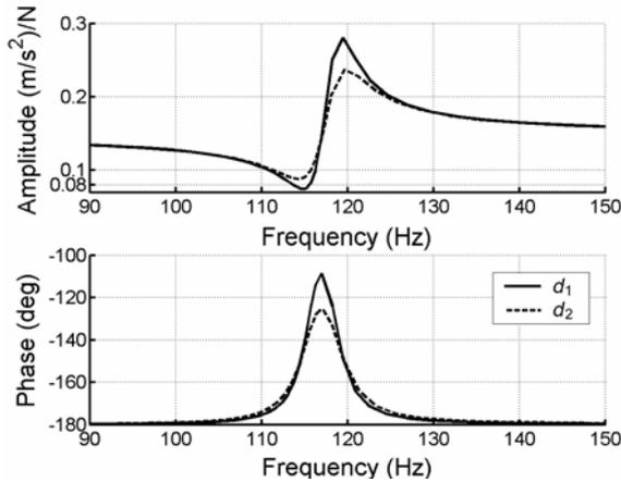
**Fig. 6:** Tuning of the damping ( $d = d_i$ ,  $d_1 < d_2$ ;  $k_e = k_1$ )
