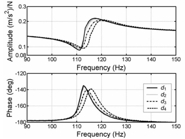
**Fig. 8:** Tuning of the damping ( $d_{\text{avc}} = d_i$ ,  $d_1 < d_2 < d_3 < d_4$ ;  $k_{\text{avc}} = k_2$ )
