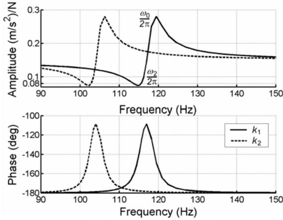
**Fig. 5:** Tuning of the stiffness ( $k_e = k_i$ ,  $k_1 > k_2$ )
