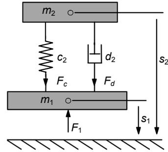
**Figure 1:** Effective mass with primary excitation and passive auxiliary mass damper
