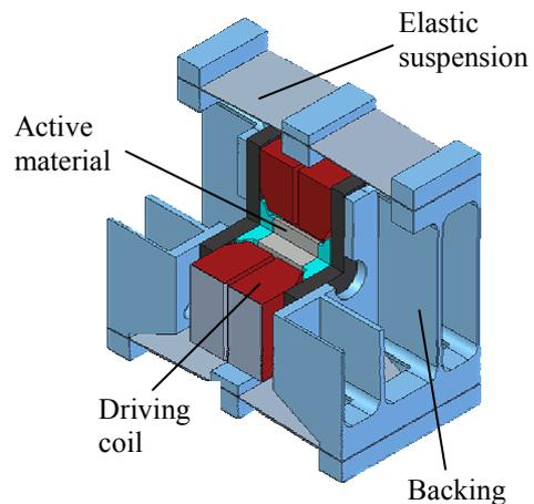
**Figure 2:** 3D model of the optimised magnetostrictive auxiliary mass damper
