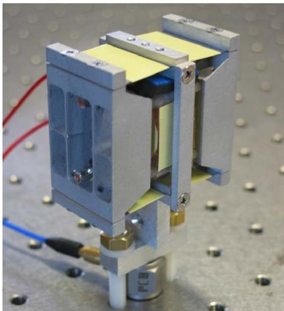
**Figure 3:** Arrangement for measuring the force generating capability
