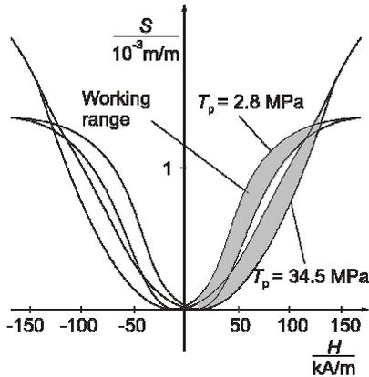
Fig. 1. Characteristics  $S(H)$  of the giant magnetostrictive material Terfenol-D under different mechanical pre-loads  $T_p$
