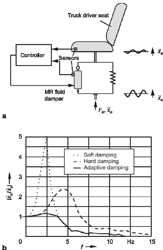
Fig. 8. MR fluid damper for driver seats: (a) system configuration; (b) vibration amplitude response [9]
