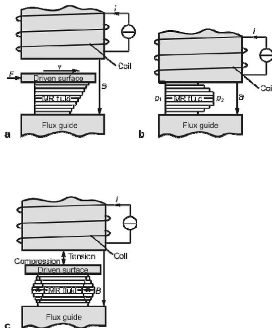
Fig. 7. Working modes of MR fluid energy transducers: (a) shear mode; (b) flow mode; (c) squeeze mode
