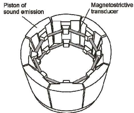
Fig. 4. Basic structure of an underwater sonar system (according to [5])
