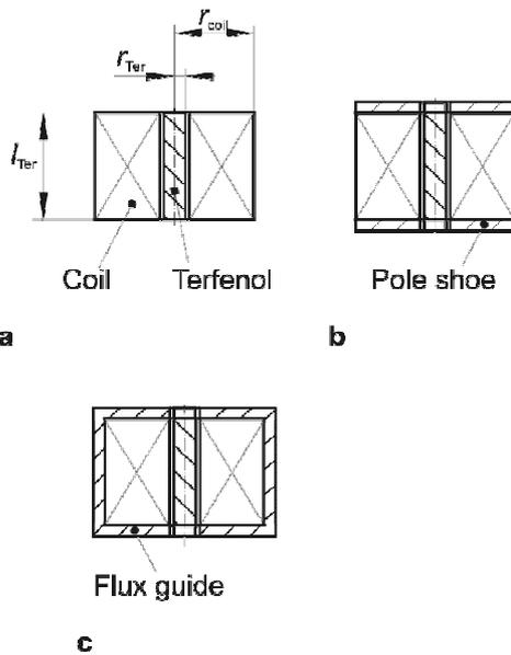
Fig. 2. Possibilities of magnetic flux guide: (a) without flux guide; (b) with pole shoes; (c) with complete flux guide
