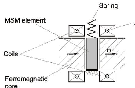
Fig. 11. Basic structure of a linear MSM actuator
